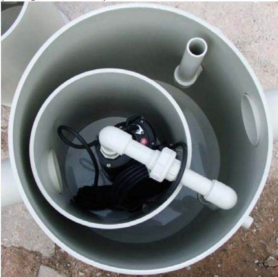
This is the Skeletank® pump sump unit with an integral overflow. The pump sits within the chamber. The pump we recommended has an internal pressure control which removes the requirement for a control panel in your house. The pump only works on demand.
